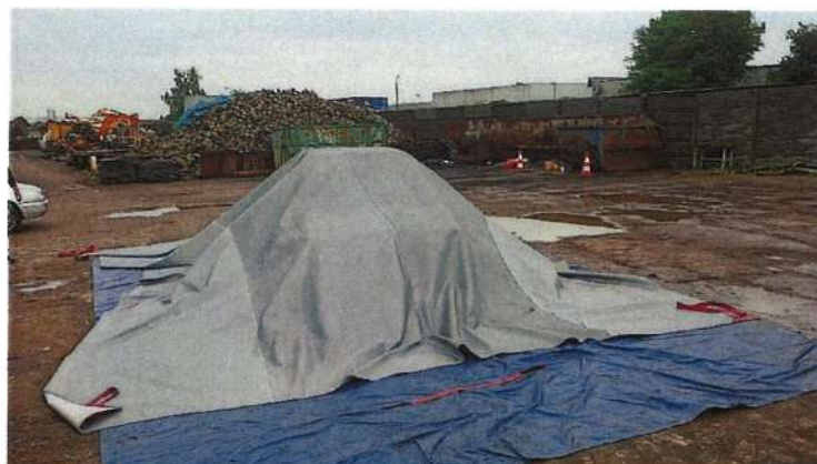
Photo 2. Fire control sheet type PG-001 applied on the vehicle Source: CNBOP-PIB.
