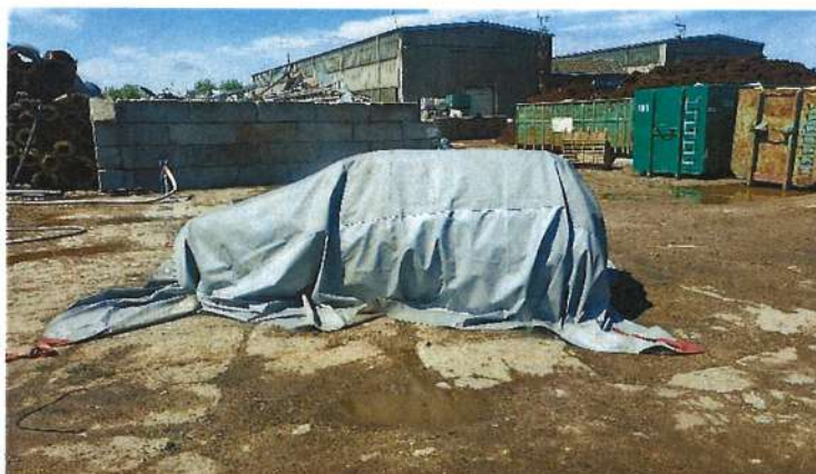
Photo. 34. Vehicle covered with vehicle fire control sheet type PG-001 Source: CNBOP-PIB.
