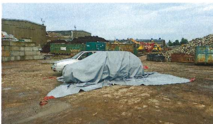
Photo. 15. Vehicle covered with the vehicle fire control sheet type PG-001 Source: CNBOP-PIB.
