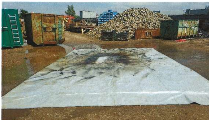
Photo. 21. Fire control sheet type PG-001 after one use and washing with water Source: CNBOP-PIB.
