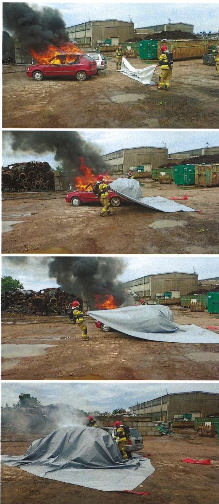
Photo. 11- 14. Placing a sheet type PG-001 over a burning vehicle
