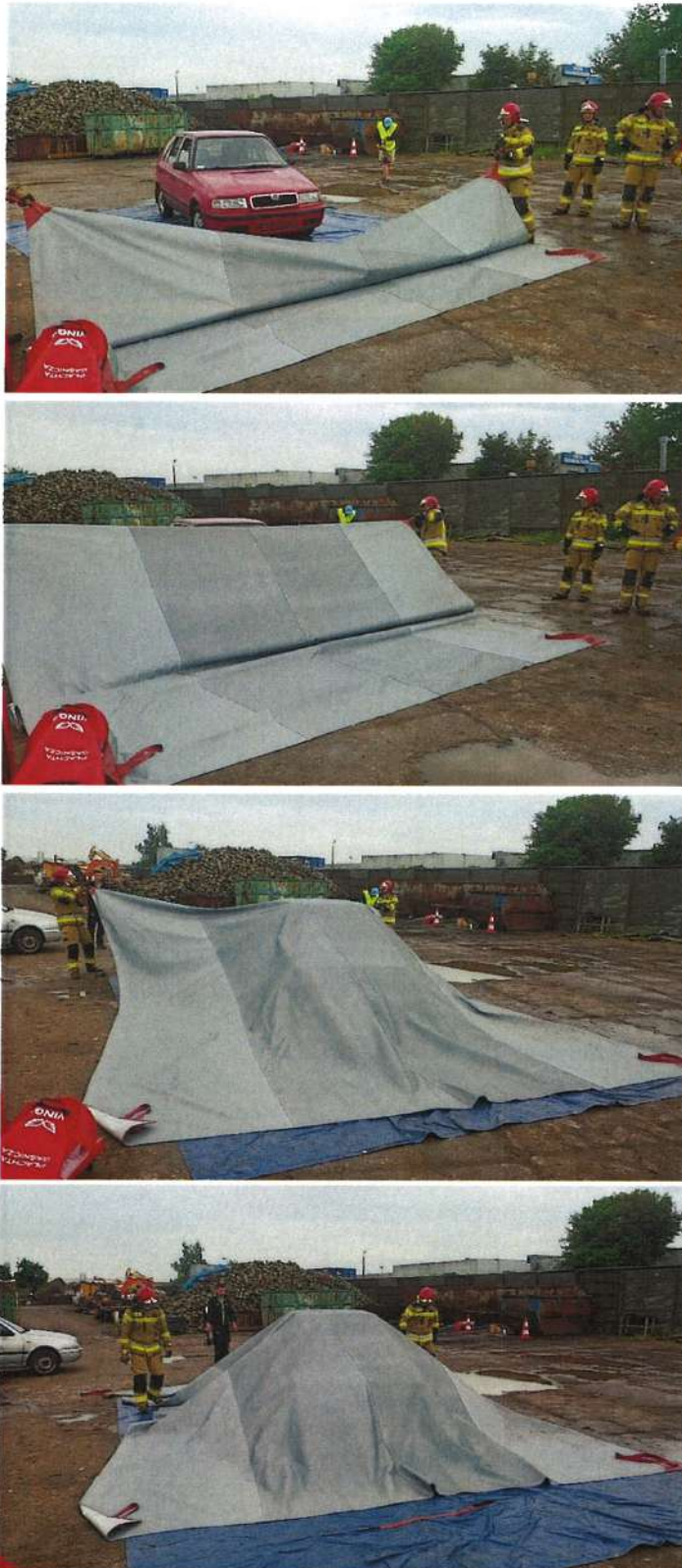
Photo. 3 – 6. Placing a sheet type PG-001 on a vehicle
